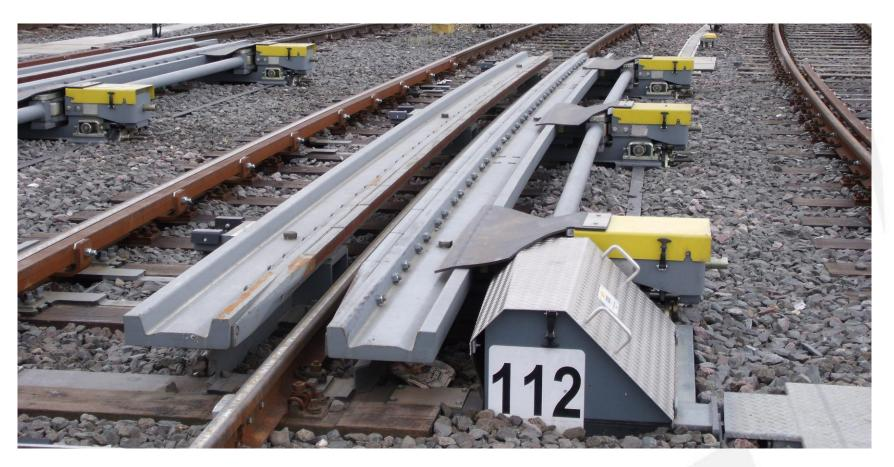
Control retarders (a kind of modern drag shoe) to brake freightwagons according kinematic models in real-time.
