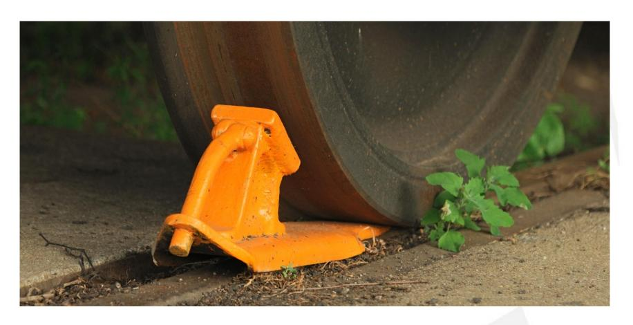
Controlling speed and distances of free running freight-wagons with drag shoe braking is a dangerous and hard job.
